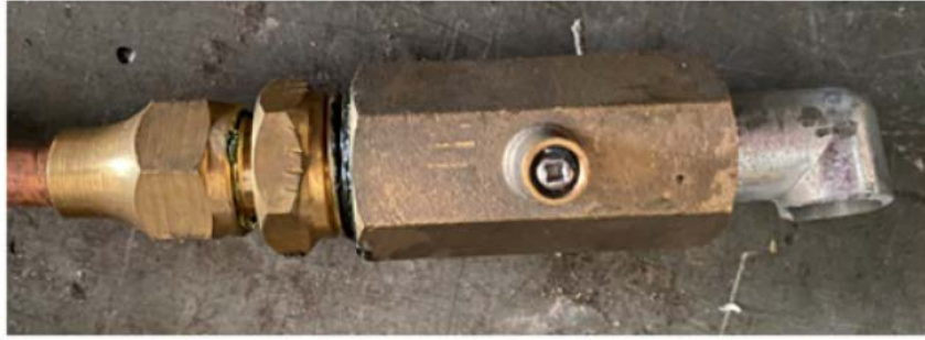
Image 2b – Failed connecting elbow in recreational vehicle
